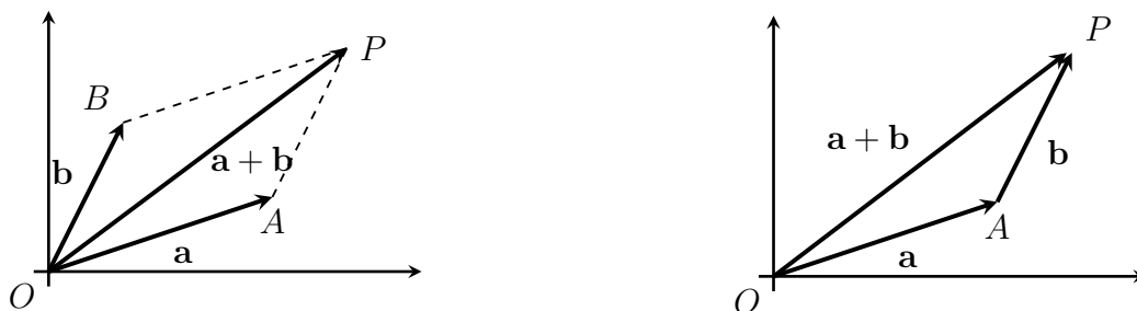
Figure 2.6: (Left) Vector addition using the parallelogram law: \mathbf{a} + \mathbf{b} represents the sum of \mathbf{a} and \mathbf{b} , which is obtained by placing the initial points of \mathbf{a} and \mathbf{b} at the same point O such that \mathbf{a} + \mathbf{b} is given by the diagonal \vec{OP} ; (Right) Vector addition using the triangle law: \mathbf{a} + \mathbf{b} represents the sum of \mathbf{a} and \mathbf{b} , which is obtained by placing the initial point of \mathbf{b} at the terminal point \mathbf{a} , such that \mathbf{a} + \mathbf{b} is given by the connection between the endpoints O and P .
