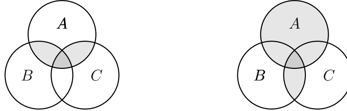
Figure 1.2: Venn diagrams showing union and intersection operations of sets: (left) (B \cup C) \cap A = (B \cap A) \cup (C \cap A) ; (right) A \cup (B \cap C) = (A \cup B) \cap (A \cup C) .
