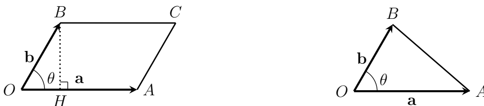
Figure 3.9: Computations of areas of parallelogram and triangle in terms of cross product: Left (parallelogram) : The vectors \mathbf{a} and \mathbf{b} are adjacent sides of a parallelogram. The angle between \mathbf{a} and \mathbf{b} is \theta . The area of the parallelogram reads |\mathbf{a} \times \mathbf{b}| ; Right (triangle) : Similarly, the area of a triangle reads \frac{1}{2} |\mathbf{a} \times \mathbf{b}| .
